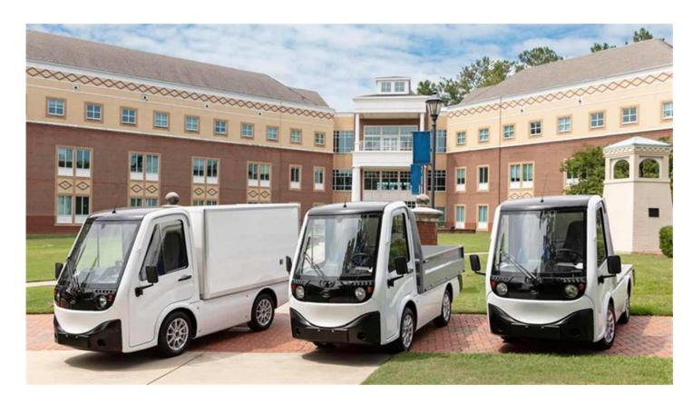
The AYRO 411 Fleet has an expected range of up to 50 miles and a maximum speed range of 25 mph (or 40 kilometers per hour), in line with the United States Department of Transportation ("USDOT") regulations for low-speed vehicles and with most state statutes, which typically limit the speed of LSVs to 25 mph on 35 mph posted roads. The current AYRO 411 Fleet includes:
