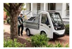
The AYRO 411 Fleet has zero gas emissions, a recharge capability of up to six to eight hours using 120V/20A outlets and has a payload capacity of up to 1,100 pounds. AYRO estimates that the AYRO 411 Fleet's operating costs are approximately 50% lower per year compared to similarly sized gas-powered trucks/vans. Vehicles in the AYRO 411 Fleet are equipped with:
